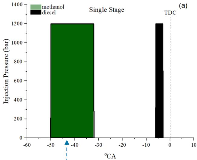
Methanol Injection During Compression
